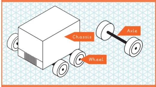
The wheels need to be attached to an axle. The axle needs to fit inside the axle holder but must not be attached to the axle holder otherwise the wheels will not turn properly.
